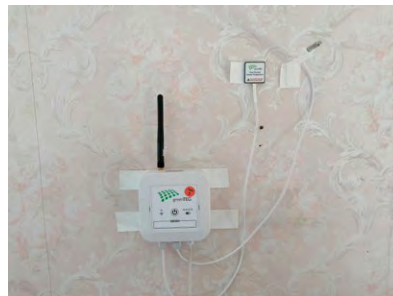
Internal GreenTEG in-situ u-value monitor installed in test apartment. © Carrig Conservation
