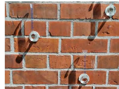
Karsten tube porosity tests underway on the historic brick of the Rubrics Building. © Carrig Conservation
