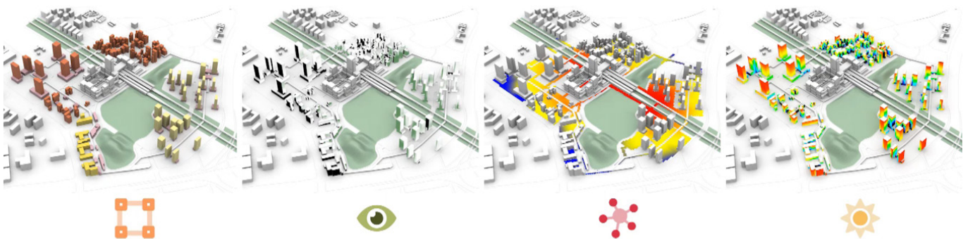
Distributed computing can run optimisation exercises on a city scale in a matter of hours. Credit: Foster + Partners
