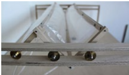
Air-actuated deployable cushion structure © Izis Salvador Pinto
