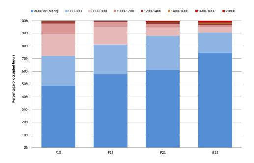
Figure 30 CO<sub>2</sub> concentration in room F13 before and after the refurbishment during winter (Before: Feb-13 – Mar-13 After: Feb-15-Mar-15)
