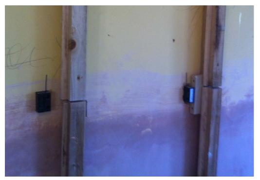
Figure 31 Moisture sensors installed on the timber studs to record moisture content
