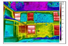
Figure 4 East elevation showing heat loss through the external wall at ground floor which is potentially due to poor insulation of the external wall
