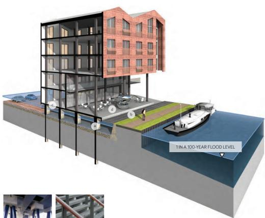
Figure 2.8a Supporting piers or posts allow flood water through
